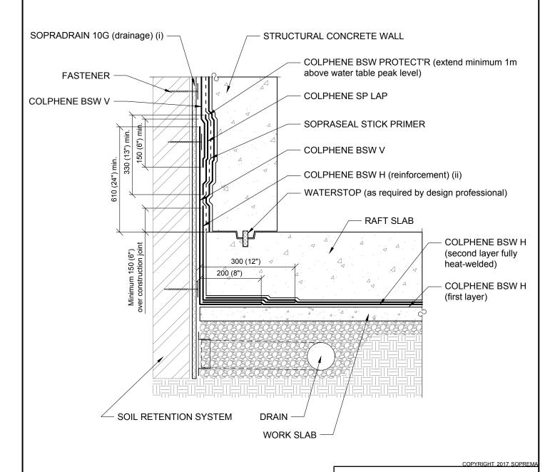
(i): Always install Sopradrain filter fabric towards soil retention system.
